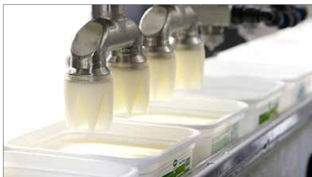
Cup filling station with drip free nozzles.
